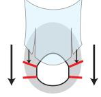
Tuck side flaps into straps. Mask worn INSIDE shield.
