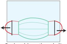
Feed mask loops through slits. Mask worn INSIDE shield.
